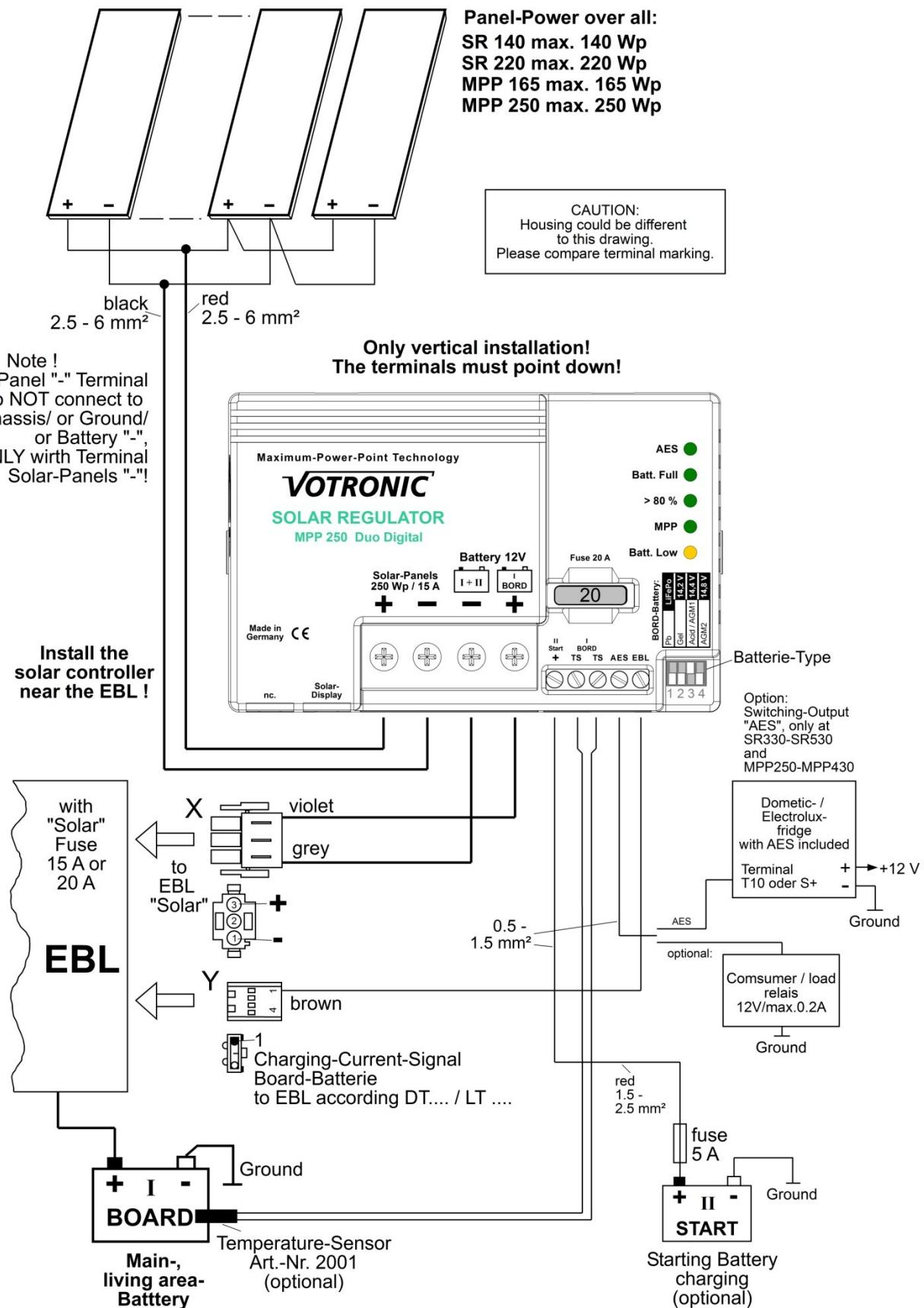
**Info:** Due to their efficiency, the SR 220 Duo Digital and MPP 250 Duo Digital can only be connected to EBL with a "solar" fuse **20 A**!
