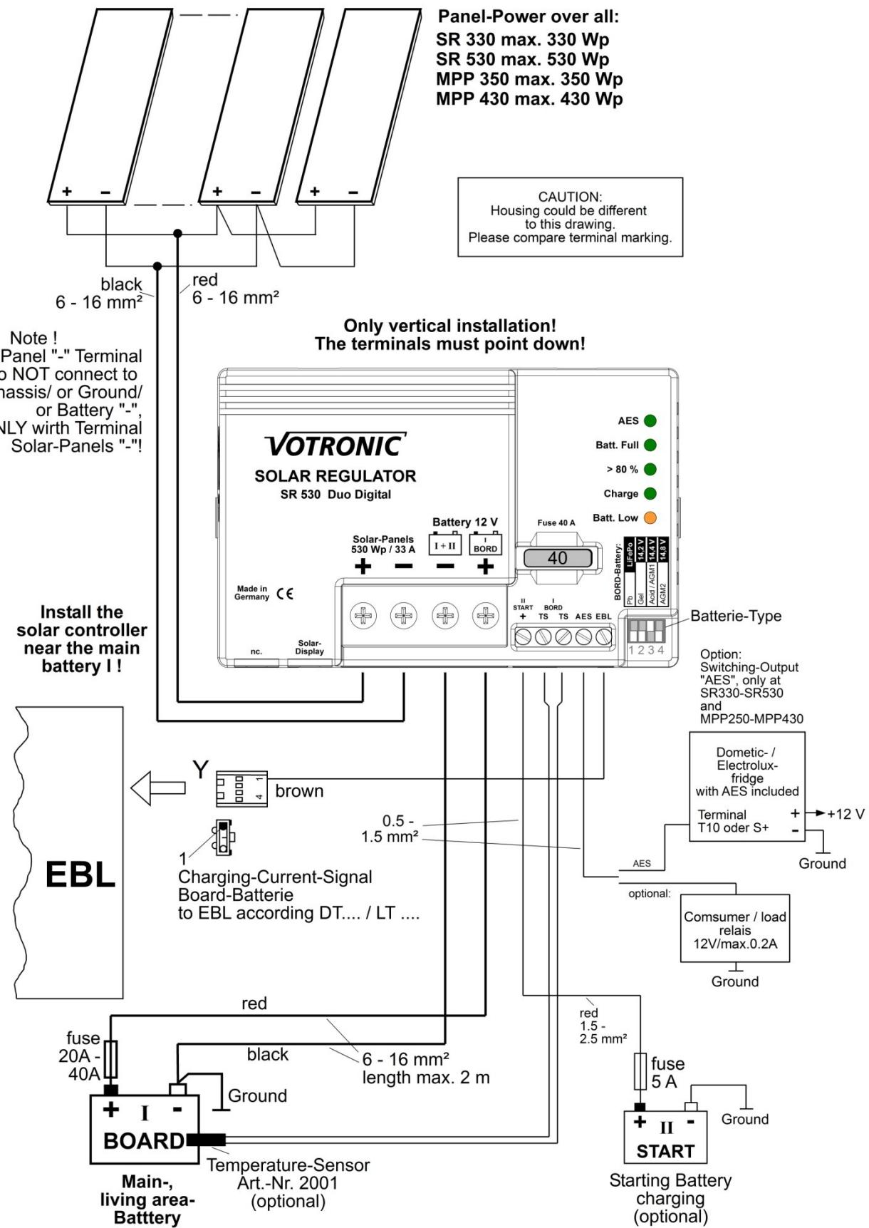
**Never lead the charging cables over the solar connection of the EBL, since eventually existing charging currents supplied by the efficient solar controllers might be too high!**
